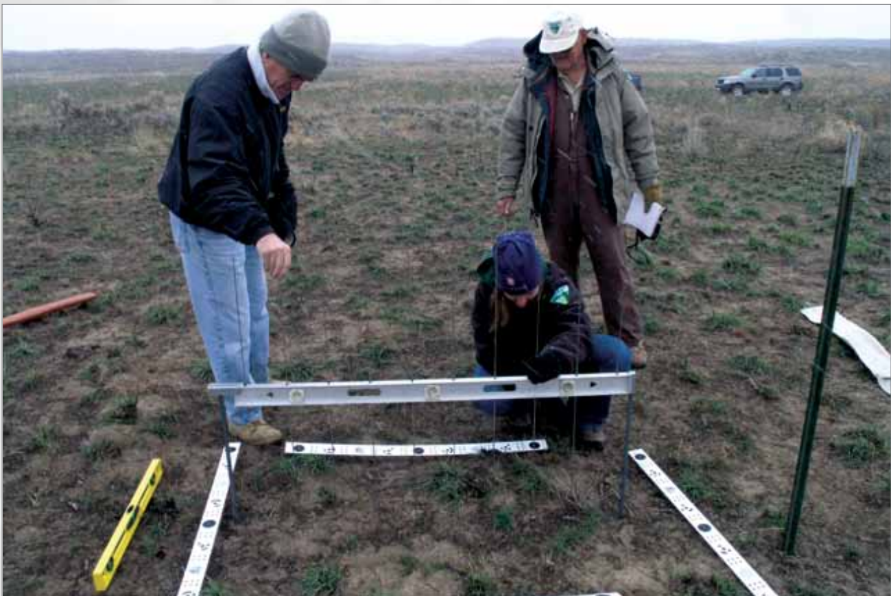
This erosion bridge is being used to determine the amount of wind erosion at a wildfire site in Idaho two years after the burn.
